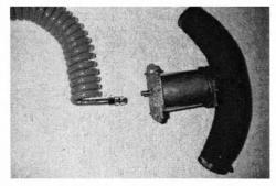
Next. you will need a good place to attach the air compressor (or some other source of air/gas pressure) to. I bought a snap-on fitting with threads and a nut at the other end and installed it in the middle of the plate that I blocked the intake with. You can of course tap into the intake system wherever you find it easy.
